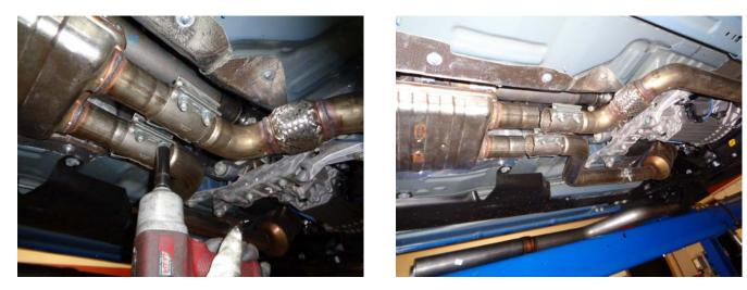
2) Support the center resonator with a stand; loosen the four nuts on the two band clamp connections at the resonator inlet. Slide the system to the rear to disengage from the clamps. See photos above.
