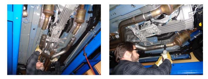
1) Place the provided 2.50" band clamps onto the front of the Scavenger assembly **26701S**, slide the assembly onto the factory head pipes approximately 3.00" and support the rear of the assembly with a stand. Be sure that the Scavenger assembly is centered in the driveline tunnel and that the embossed Flowmaster in the center case is facing the ground. Tighten both band clamps enough to hold, but still allow for adjustment.
