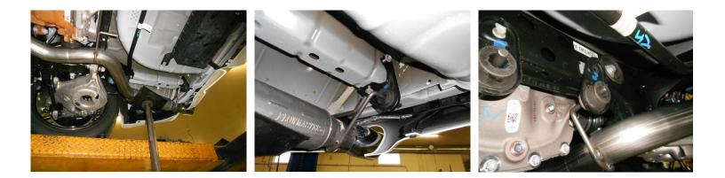
4) Place the right muffler assembly **#815430-487** up into position and slide the inlet completely onto the **26703S** mid pipe. Support the assembly with a stand and remount the rear hanger mount to the frame, tighten securely. Remount the front hanger to the cross member and tighten securely. Leave the clamp on the inlet loose for now. Repeat this step with muffler assembly **#815430-488** on the left side of the vehicle.
