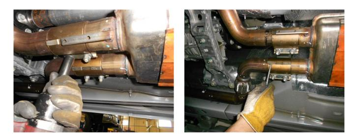
5) Support the center resonator with a stand and loosen the four nuts at the two band clamp connections at the resonator inlet. Using a screwdriver, pry up the clips on the clamp body to release the clip from the tab on the inlet pipes. Slide the clamp assemblies slightly back to clear the tabs. You can now lower the rear of the resonator and slide the assembly to the rear of the vehicle to remove. Lower the resonator from the vehicle and set aside.
