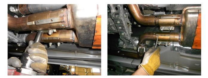
4) Loosen the four nuts at the two band clamp connections at the inlet of the center resonator. Using a screwdriver, pry up the clips on the clamp body to release the clip from the tab on the inlet pipes. Slide the clamp assemblies slightly back to clear the tabs. With the help of an assistant, carefully lower the stand and slide the assembly back to disengage from the inlet pipes.
