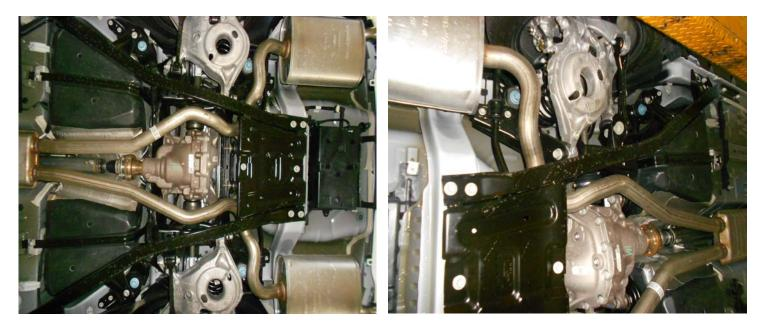
1) The body braces shown in the photos above will need to be removed in order to remove the factory system and install the Flowmaster system. Starting at the front of the right side (passenger) brace, loosen the front bolt and then work your way to the rear of the vehicle removing the next eight bolts, lower the brace from the vehicle. Repeat this step on the left side of the vehicle with the six bolts on that side.
