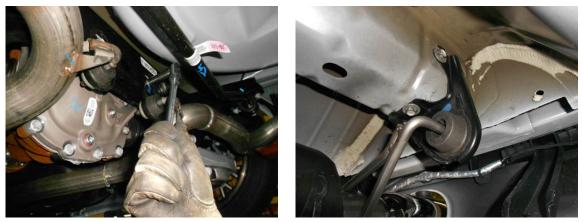
3) Using a 13mm wrench, loosen the two hangers just behind the rear differential from the cross member and the two hanger mounts at the rear of the vehicle from the frame. Slide the muffler assemblies toward the rear of the vehicle to disengage them from the factory system. Leave them hanging in place for re-assembly onto the Flowmaster X-pipe assembly.
