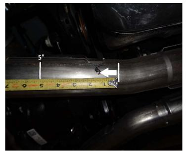
4) Measure back 5" from the beginning of the straight area marked in the previous step and make a mark on both pipes as shown in the photo at left. Support the exhaust system both in front and behind the area to be cut. Check that the marks are correct, then using a sawsall, cut both pipes at the marks. Note: Due to the closeness of the pipes to the gas tank, use caution when cutting! Carefully deburr the end of the muffler inlet pipes where cut with a file or die grinder.
