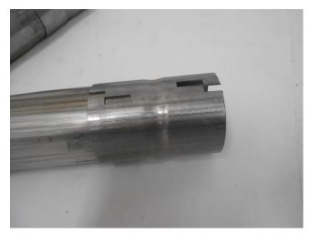
1) Slide the supplied **TB809S** adapter pipes onto the end of each outlet of the **86480S** X-pipe assembly. Place a supplied clamp onto the connections and tighten enough to hold.
