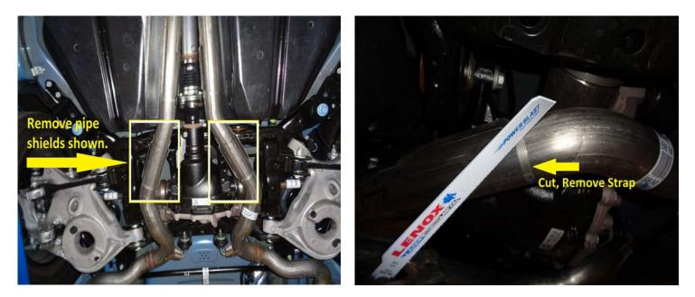
2) Begin by removing the two pipe heatshields indicated in the first picture above. Cut thru the strap at the rear of the shield, then lift and lower the shield a few times to break the weld at the front of the shield. Remove.
