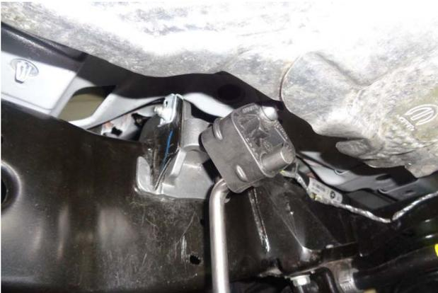
14. Put the factory hanger mounts into position, then reinstall and tighten the factory bolts.
