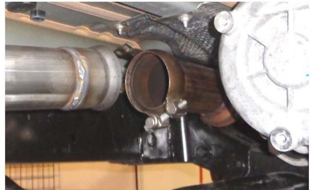
11. Slip the factory clamp over the ball end of the factory pipe, mate the front end of **front pipe 86500S** to it, then snug the clamp just enough to still allow adjustment. Rotate the pipe so that it is level and parallel to the vehicle frame.
