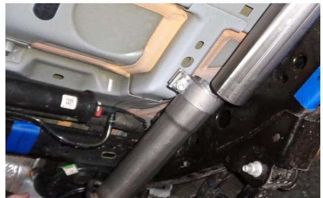
12. Slip a **clamp MC250BS** over the front end of **rear pipe 86501S**, then slide the pipe over the rear of the front pipe while pushing the pipe's hanger into the rubber mount on the vehicle. Snug the clamp just enough to still allow adjustment.
