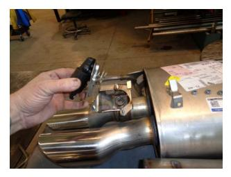
3) Lift the actuator with the heatshield and spring attached from the factory valve assembly.
