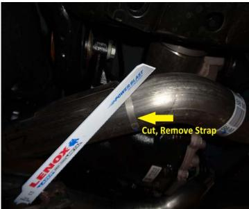
3) Begin by removing the two pipe heatshields indicated in the first picture above. Cut thru the strap at the rear of the shield, then lift and lower the shield a few times to break the weld at the front of the shield. Remove.
