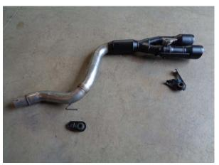
1) Place the new Flowmaster muffler units next to the factory units and swap the front and rear hanger mounts from the stock mufflers to the new mufflers. Also, place a provided 2.50" clamp onto the inlet of each assembly. Tighten the clamp just enough to hold in place.
