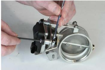
6) Use the remaining ¼" hardware to secure the actuator to the mount in the remaining two holes. Tighten securely using a 7/16" open end and 5/32" Hex wrench.
