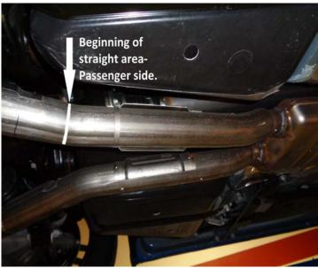
4) Behind the factory center resonator, follow the pipes back just past the second bend of each pipe, make a mark on each pipe where the bend ends and the straight area begins. See above photos. At the rear of each muffler unplug the wire to the factory exhaust actuator and tuck the connection up out of the way until ready to re-connect to the new mufflers.
