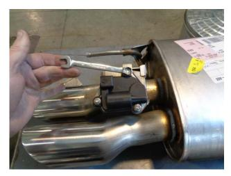
2) On the factory mufflers, use a 10mm wrench to remove the three nuts securing the exhaust valve actuator to the exhaust valve. Place the three nuts and the grounding clip aside for re-installation on the new Flowmaster mufflers.
