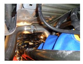
1) Place the supplied clamp onto the inlet of the new tailpipe, then place the pipe up into position and slide onto the factory over-axle pipe. Line up the notch in the pipe with the tab on the over-axle pipe, slide on completely. Support the pipe with a stand if necessary.
