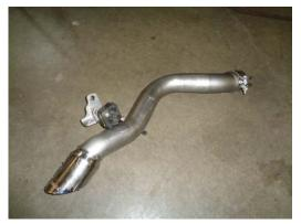
5) Place the factory muffler next to the new Flowmaster High clearance tailpipe assembly and move the drivers side hanger mount from the muffler onto the wire hanger of the new pipe.
