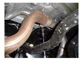
2) Support the muffler with a stand, then using a 15mm socket, loosen the clamp at the muffler inlet connection above the rear axle.
