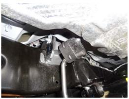
2) Place the factory hanger mount back into position on the frame and secure using the factory bolts, tighten securely.
