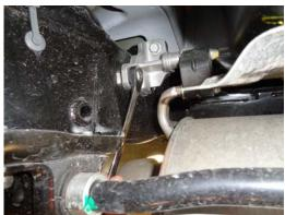
3) Locate the left and right rear mounts supporting the muffler, use a 13MM open end wrench to remove the lower bolt on each mount.
