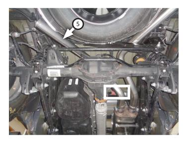
14. Place **clamp (8)** onto **left exit (6)** inlet. Connect left exit to left over-axle and hang wire hanger in stock isolator. Tighten clamp just enough to allow for adjustment.
