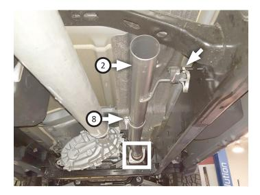
11. Connect ground wire to mount. Place **clamps (x3) (8)** on **muffler (3)** inlet and outlets, then connect muffler to extension. Tighten clamp on muffler inlet just enough to allow for adjustment.
