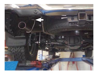
15. Place **tips (x2) (7)** onto exit tailpipes and tighten inlets. Rotate exit pipes and tips to desired distance from body or bumper, so angle cut on tips are properly positioned.
