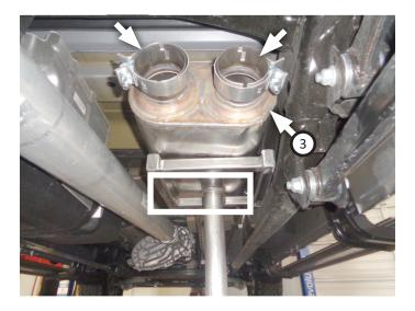
12. Thread **right tailpipe (4)** over axle and hang rear wire hanger in stock isolator. Connect right tailpipe to muffler and hang front wire hanger in stock isolator. Tighten clamp just enough to allow for adjustment.
