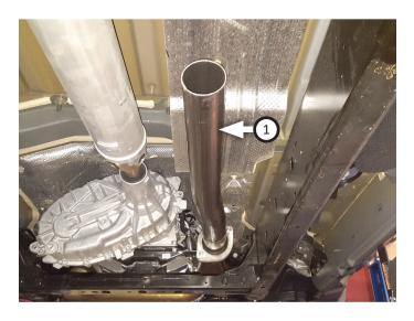
Fasten inlet with (x2 ea) bolts (9), flat washers (11), lock washers (12) and nuts (10). Place clamp (8) onto extension (2) and connect it to inlet pipe. Insert hanger in isolator then tighten clamp to allow for adjustment.
