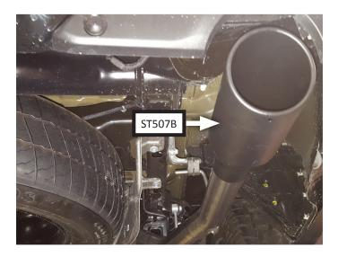
Place tip (ST507B) onto left tailpipe. Tighten inlet to secure connection.
