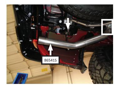
Place 2¼" clamp (MC225BS) onto right tailpipe (86540S). Connect left tailpipe to left exhaust outlet and insert wire hanger into isolator. Tighten clamp just enough to allow for adjustment.
