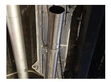
14. Place clamp (MC350BS) onto muffler (8535562-Z) inlet. Place clamps (x2) (MC250BS) onto muffler outlets. Connect muffler to inlet or extension pipe then tighten front clamp just enough to allow for adjustment.
