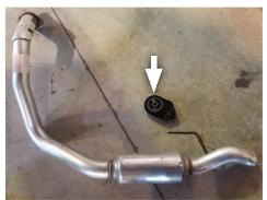
7. Remove passenger side tailpipe isolater from frame. Then cut remaining tailpipe assembly just behind muffler exit.
