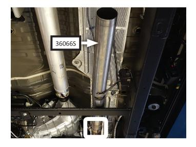
13. Place **clamp (MC350BS)** onto **extension pipe (36065S)** inlet then connect extension to inlet pipe.
