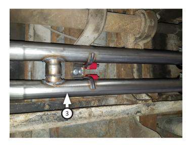
11. Place (x2 ea.) clamps (13) onto mufflers (4) then connect them to h-pipe assembly. Tighten clamps just enough to allow for later adjustment. Place (x2) clamps (13) onto end of mufflers.
