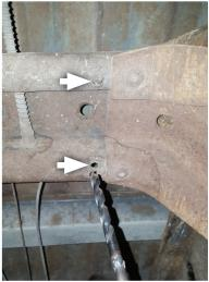
8. Mark line on front crossmember  $2\frac{1}{4}$ " outward from tank bracket as shown. Use **front frame hanger (12)** oriented as shown to drill (x2)  $\frac{1}{4}$ " mount holes.
