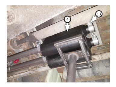
12. Hang (x2) **front hangers (15)** on front of **left (5)** and **right (6)** tailpipes. Hang (x2) rear hangers (step 6) onto rear of left and right tailpipes.
