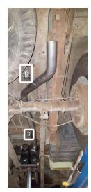
14. Route left tailpipe over axle and connect it to muffler. Fasten front and rear hangers to vehicle frame with (x3) bolts (17), (x6) flat washers (19), (x3) lock washers (20) and (x3) nuts (18).
