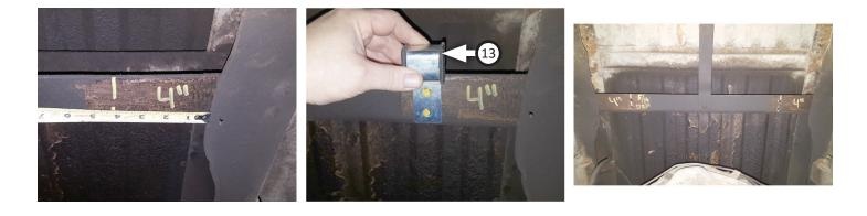
**NOTE:** For short bed vehicles only, trim 16" from rear of H-pipe for proper fit.
