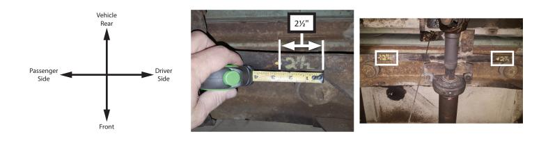
Use (x2) rear frame hangers (14) (oriented flanges out) to drill <sup>5</sup>/<sub>6</sub>" mount holes then install hangers with (x2) bolts (15), (x4) flat washers (17), (x2) lock washers (18) and (x2) nuts (16).
