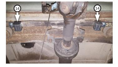
Mark rear cross member on both sides, inboard 4" from intersecting frame edge. Use (x2) rear hangers (13) oriented as shown to center then drill mount holes.
