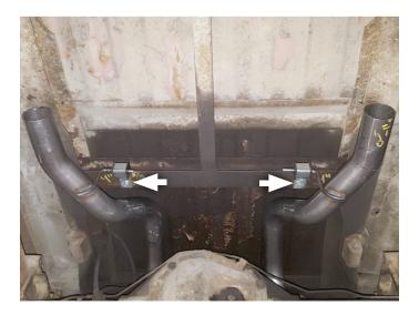
Secure (x2) front hangers (on tailpipes) to crossmember (step 10) with (x2) bolts (15), (x4) flat washers (17), (x2) lock washers (18) and (x2) nuts (16).
