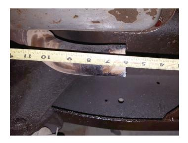
5. Mark forward cross member on both sides, inboard 2<sup>1</sup>/<sub>2</sub>" from intersecting frame edge.
