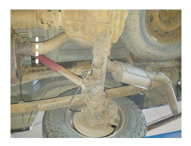
4. Support muffler and disassemble wire hangers from isolators. Loosen band clamp, disconnect inlet pipe then remove exhaust system.
