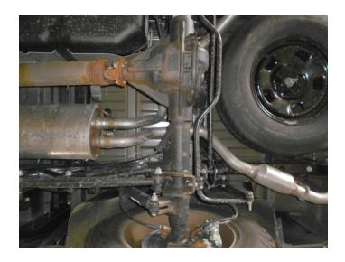
4. Disassemble wire hangers from isolators on muffler and inlet, then remove clamp on slip connection behind factory Y-pipe. Remove muffler and set aside.
