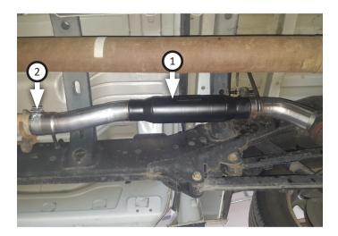
7. Recommended: Secure slip-fit connection with a 1-inch tack weld then spray high-temp paint over weld to prevent rust and premature corrosion.
