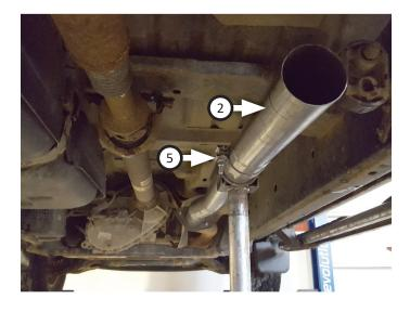
Remove muffler hanger mount, slide it onto muffler (3) and place clamp (5) onto muffler. Connect it to inlet/ extension, insert hanger into isolator then fasten hanger mount into place on frame.
