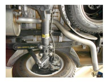
4. Support muffler and disassemble wire hangers from isolators. Remove and retain (x2 ea.) flange nuts and bolts, disconnect inlet pipe and remove exhaust system.
