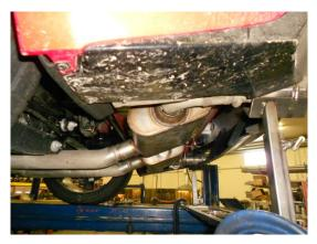
2) Place the inlet of muffler **8425461** onto the factory front pipe and support with a stand. Connect the factory exit pipe to the outlet of the muffler. Adjust the position of the muffler and exit pipe to get a satisfactory fit. Be sure that the exit pipe is in the correct position in the bumper cut-out. Once you are satisfied with the position of the muffler and exit pipe, fully weld the inlet and outlet of the muffler. Repeat this step on the opposite side of the vehicle.
