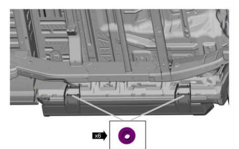
3. Remove the running board assembly.
