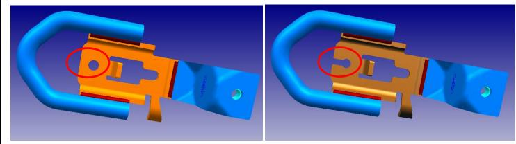
Re-install 4x bolts from Step 3 Torque: 62.5 +/- 9.4 Nm Install 4x bolts supplied with kit Torque: 80 +/- 12 Nm
