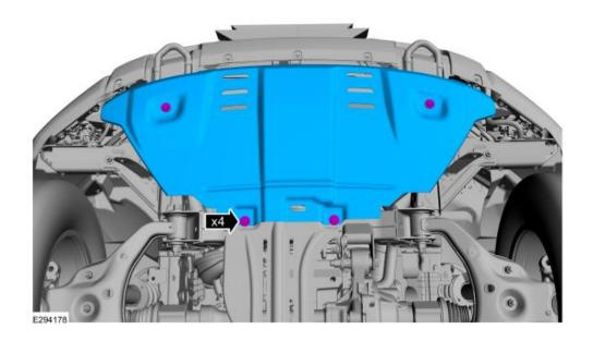
3. If equipped, remove the bolts and the front bumper air deflector. *Torque*: 28 lb.in (3.2 Nm)
