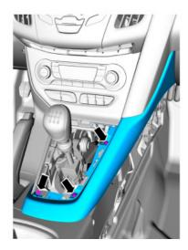
STEP 3: Remove push pin from left side panel. Pull on panel to release the 5 remaining attachment points. (See figure below)
