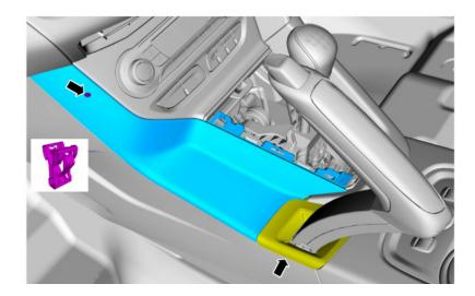
STEP 5: Remove push pin from right side panel. Pull on panel to release the 2 remaining attachment points. (See figure below)
