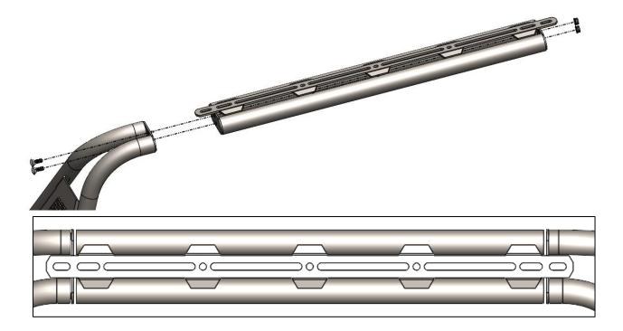
**<u>Step 2</u>**: With additional help, carefully place Sport Bar onto bed rails aligning edge with the plastic cap on both sides.
