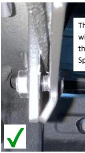
The lip of the bed cap will sandwich between the backing plate and Sport bar.
