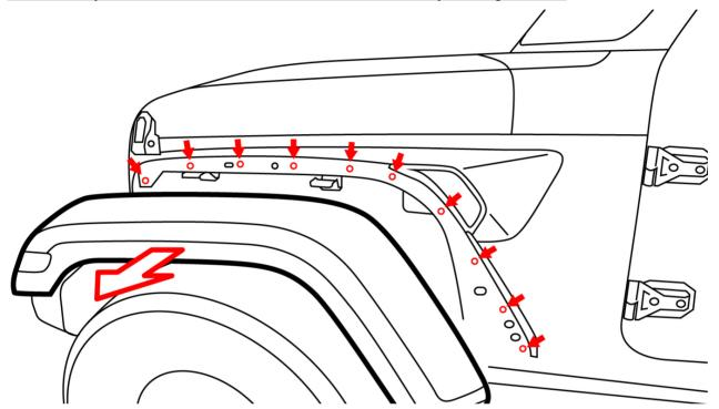
2. Locate factory wiring harness and feed wires: Locate the wiring harness and unplug. Set the fender aside for now. You will use THIS harness to tap the XK Fender Vent Light into. Remove the existing fender vent by using body clip removal tool. Feed the XK Fender Vent wiring through the large top hole (as highlighted with bold red line below) in the body of the vehicle behind the Fender Vent.
