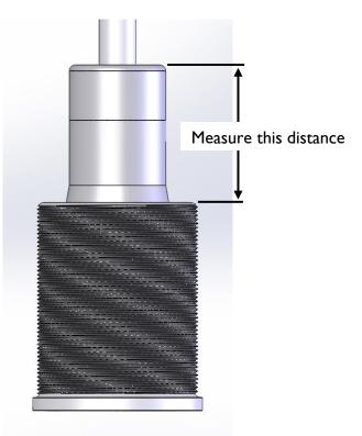
8. Locate the D112-0072 Dinan Shock Cap and D671-0223 O-ring in the hardware kit. Insert the O-ring into the groove inside the cap, and install cap onto shock. If needed, add a small amount of lubricant to ease assembly.
