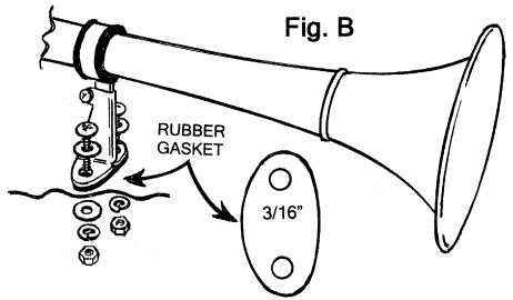
IMPORTANT: Make sure the hole is free of any burrs that could cut into the horn's wire. For roof mount mounting, to prevent water leaks, it is recommended that silicon or a waterproof sealer be placed on the wire at the point of entry into the roof
