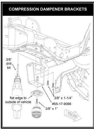
Drill the two marked locations using a 3/8" drill bit. Also drill-out the mounting hole in the factory compression stop cup to 3/8".
