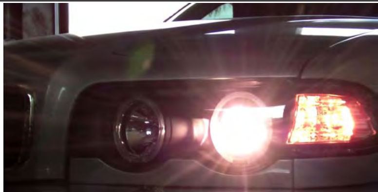
Spyder Projector Headlight using Factory Xenon Lights
