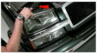
1) Open the hood. Remove the headlight retainer stake by sliding it out towards the grille.
