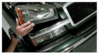
2) Unseat the headlight and disconnect the headlight wiring harnesses.
