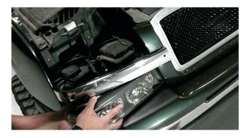
5) Reinstall the DRL socket and turn signal socket into the SPYDER lower lens assembly, then seat the lower lens assembly.
