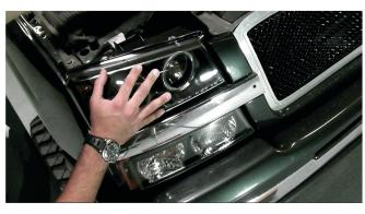
6) Reconnect the OEM headlight harness to the SPYDER upper lens Projector headlight assembly. Seat the SPYDER upper headlight lens.
