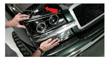
7) Reinstall the headlight retainer stake to secure the upper headlight lens assembly.
