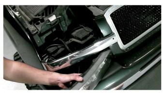
4) Unseat the lower lens assembly and disconnect the DRL socket and turn signal socket, then remove the lower lens and set it aside.
