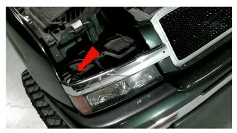
3) Remove the headlight. Squeeze the tab indicted to loosen the lower lens assembly.
