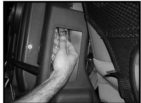
2. Remove the torx nut from the bottom of each factory hinge pin. Set these nuts aside to be re-installed on the Tube Doors. To remove the factory doors, carefully lift the door upward until the hinge pins completely clear the hinges. It will be helpful to have someone else assist with this step.
