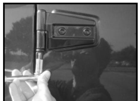
3. To install Tube Doors, lightly lubricate the tube door hinge pins. Position the hinge pins directly above the hinges. Slowly lower the hinge pins into the door hinges. If the hinge pins do not fully seat, slowly rotate the door back and forth until hinge pins fully engage. Install torx nuts removed in the previous step.
