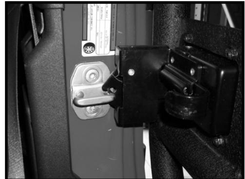
5. Attach the loop of the Adjustable Nylon Strap to the hook on the Tube Door and the hook inside the vehicle. By using different loops to attach to the vehicle hook, the amount of door opening can be adjusted.
