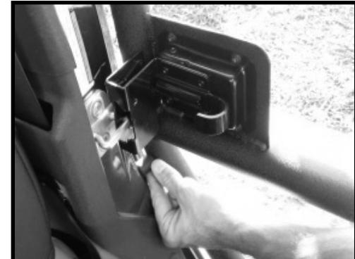
2. Drill a 3/32" hole and attach the bumper with the supplied sheet metal screw. Do not overtighten. The attachment screw can be loosened or tightened as necessary to adjust the length of the Anti-Rattle Bumper.
