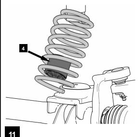
INSTALL THE BUMPSTOP ONTO THE AXLE
