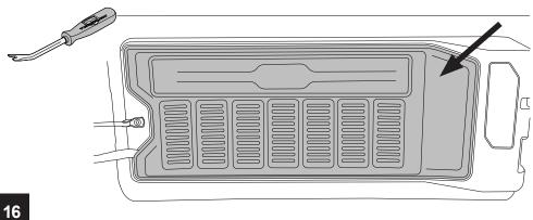
**NOTE: WHEN** PANEL IS REMOVED SOME RETAINERS MAY STAY IN THE DOOR. REATTACH **RETAINERS TO** PANEL BEFORE REINSTALLING.
