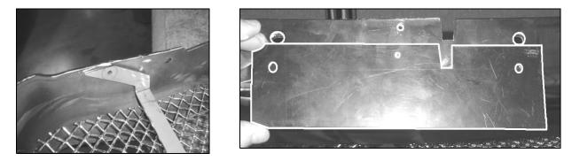
**<u>STEP 6:</u>** Locate the provided template. Place the template on the out side of the grille lined up with the two holes and notch on top of the grille (5). Drill the third hole in the top using this template. Place the last bracket on the inside of the shell. Using the Machine screw and washer, place it through the shell into, the bracket and into the nylon lock nut. Making sure that the mesh lays flat, tighten the hardware.
