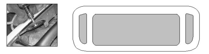
**<u>STEP 4</u>**: Now test fit the mesh in the grille to see if more material will need to be trimmed around the chrome ring. Place the grille face down on a table. Center the mesh in the shell. The mesh should fit flush along the lower and side edges so there is no gap between the mesh and the chrome ring (If it does not, trim the needed areas).
