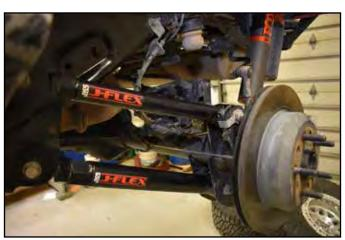
O Mount the control arm to the frame bracket with the grease fitting up. Install the original mounting bolt and flag nut. Finger tighten the bolt. DO NOT torque mounting hardware until instructed.
