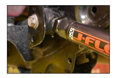
HINT: If mounting bolt is difficult to install due to misalignment of Control Arm bushing with mounting bracket, either (1) adjust height of axle housing with hydraulic jack, (2) move axle housing into position with a heavy-duty ratchet strap, or (3) temporarily disconnect track bar until mounting holes align.
