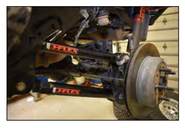
Mount the control arm to the frame bracket with the grease fitting down. Install the original mounting bolt and flag nut. Finger tighten the bolt.
