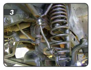
Note: If difficult to remove the sway bar link from the sway bar, an air chisel or pickle fork can be used.
