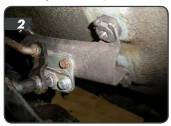
Check transfer case shift operation to see that all positions engage completely. Adjust the shift linkage as necessary. The linkage adjustment is located near the pivot bracket.
