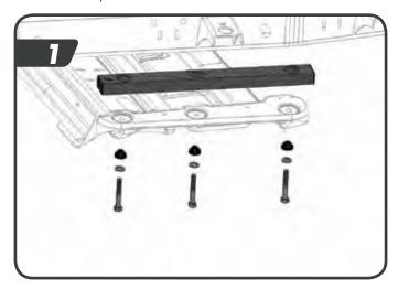
Repeat the transfer case drop tube installation on the passenger side.
