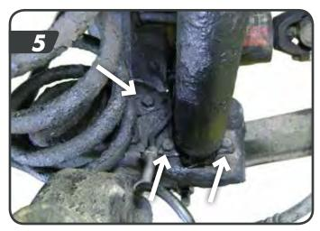
Remove the front lower control arms from the vehicle. Save hardware.
