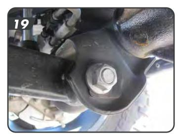
e. Repeat cam bolt installation on the driver's side.
