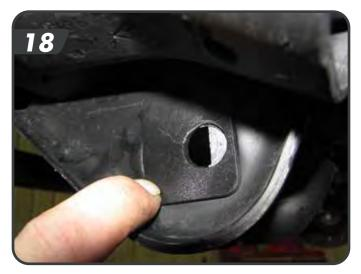
d. Re-install the control arm to the axle with the factory bolt with cam lock washers. Rotate the cam lock so that the bolt will be as far back in the slot as possible (most rearward setting = max caster). Snug the cam hardware so that the cams are retained within the stops. Final torque will be completed with the weight of the vehicle on the suspension. [19]
