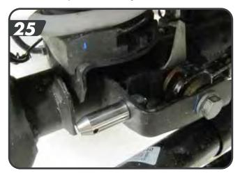
s. Install the longer disconnect post on the driver side axle sway bar link mount with it pointing inboard [26]. Fasten with the ½" nylock nut and tighten to 64 ft-lbs. Tighten the post with the pin hole parallel to the ground. Slide the polyurethane spacer on the pin up against the axle tab.
