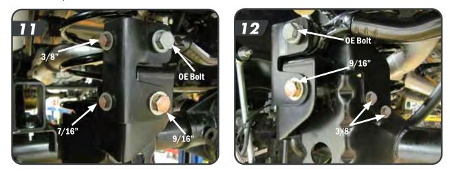
q. Drill the holes and fasten the bracket to the axle with the provided hardware. Insert the provided sleeve in the OE track bar position.
