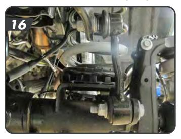
h. Remove the 4 bolts mounting the front driveshaft to the pinion flange (15mm). This is done to ensure the driveshaft does not bind when removing the coil springs. [17]
