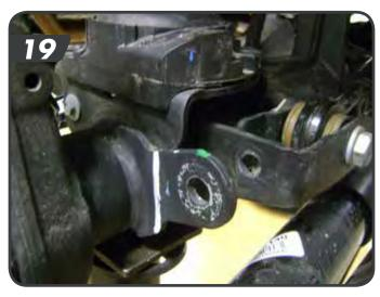
Install the shorter passenger side post on the side of the track bar mount at the sway bar link mount location with it pointing outboard [19]. Fasten with the ½" nylock nut and tighten to 65 ft-lbs.
