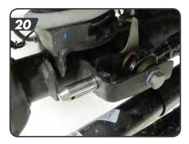
Install the longer disconnect post on the driver side axle sway bar link mount with it pointing inboard [20]. Fasten with the ½" nylock nut and tighten to 65 ft-lbs. Tighten the post with the pin hole parallel to the ground. Slide the polyurethane spacer on the pin up against the axle tab.
