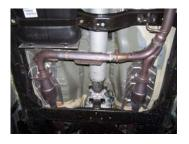
2. To remove the stock exhaust, unbolt the 2-bolt flanges located in front of your factory muffler. Next, unbolt your stock tailpipe behind your muffler. Do not discard your factory hardware, you will reuse it. (May need to remove spare tire for easier removal of tailpipe.)
