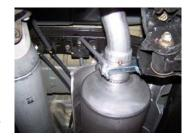
6. Next, install rear muffler hanger #F onto outlet of muffler. Insert hanger into rubber grommet. Do not tighten.
