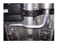
3. Install Y-pipe #A onto your existing stock flanges. Insert hanger into rubber grommet. Use your factory hardware to secure. Do not tighten.
