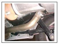
LAY OUT THE GIBSON EXHAUST ON THE FLOOR AND COMPARE PART #'S TO THE DRAWING. TO REMOVE YOUR FACTORY EXHAUST UN-BOLT YOUR TAILPIPE AT THE CLAMP LOCATED BEHIND YOUR STOCK MUFFLER USE WD-40 TO AID YOU IN REMOVAL OF HANGERS FROM RUBBER CDUMMETS
