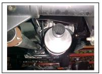
INSTALL MUFFLER # C ONTO YOUR RESONATOR 1 1/2" -2". USE CLAMP #G TO SECURE MUFFLER TO THE PIPE, DO NOT TIGHTEN. OUTLET WILL BE AT THE 12 O'CLOCK POSTION. INLET WILL BE LOOKING INTO LOUVERS.
