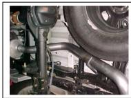
**INSTALL OVERAXLE** TAILPIPE # D INTO MUFFLER 1 1/2"-2" INSERT WELDED HANGER INTO RUBBER GROMMET USE CLAMP # G TO SECURE PIPE TO MUFFLER.
