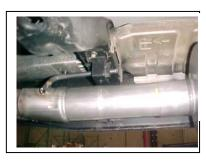
NEXT, INSTALL RESONATOR # B 1 1/2"-2" ONTO Y-PIPE USE CLAMPS # G TO SECURE PIPES TOGETHER, DO NOT TIGHTEN.
