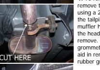
1. To remove the stock exhaust remove the nut on the rear hanger using a 21mm wrench, then cut the tailpipe just after the rear muffler hanger and remove. Unbolt the headpipe at the flange and remove. Leave all rubber grommets in place. Use WD-40 to aid in removal of hangers from rubber grommets.
