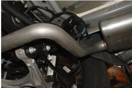
5. Install the Passenger side muffler assembly onto the factory pipe and into the factory rubber grommets. Do not tighten.
