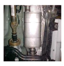
LAY OUT THE GIBSON EXHAUST ON THE FLOOR SO IT LOOKS LIKE THE DRAWING AND COMPARE IT TO THE MANUAL. TO REMOVE THE STOCK EXHAUST CUT OFF TAILPIPE JUST BEHIND THE MUFFLER THEN REMOVE MUFFLER FROM 2- BOLT FLANGE JUST IN FRONT OF MUFFLER, LEAVE ALL RUBBER GROMMETS IN PLACE, USE WD-40 TO AID IN REMOVAL OF EXHAUST AND HANGERS.
