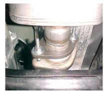
ATTACH MUFFLER ASSEMBLY #A ONTO YOUR EXISTING STOCK FLANGE. USE BOLT KIT # E TO SECURE TO FLANGE. USE A JACK STAND TO SUPPORT THE MUFFLER.
