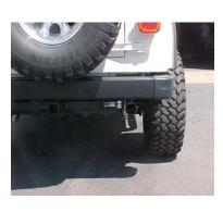
INSTALL STAINLESS STEEL TIP. CLAMP DOWN. WHEN YOU HAVE EVERYTHING IN PLACE, FIRMLY TIGHTEN ALL BOLTS AND CLAMP DOWN SECURELY. TO CLEAN STAINLESS TIP, USE A SCOTCH BRITE PAD AND ANY STAINLESS STEEL OR ALUMINUM CLEANER.
