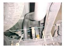
INSTALL OVERAXLE TAILPIPE # D INTO THE MUFFLER, ATTACH CLAMP # E. DO NOT TIGHTEN
