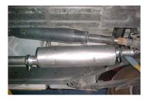
THEN INSTALL THE MUFFLER ON HEADPIPE #A NO LESS THAN 1-1/2" TO 2" USING CLAMP #E. THE MUFFLER OUTLET WILL BE CLOCKED AT 12 O'CLOCK POSITION. INLET OF MUFFLER HAS LOUVERS FACING THE MOTOR. DO NOT TIGHTEN.
