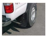
INSTALL THE STAINLESS TIP. USE A STAINLESS STEEL OR ALUMINUM CLEANER AND ANY SCOTCH BRITE PAD TO CLEAN. NOW TIGHTEN ALL HANGERS AND CLAMPS.
