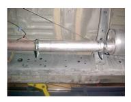
Install head pipe # A on to your existing stock front pipe and secure with clamp # G.
