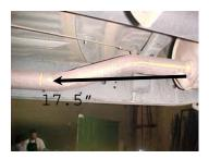
Lay out the exhaust on the floor so it looks like the drawing and compare parts with manual. **To remove the stock exhaust Cut it 17 ½" in front of the muffler.** Leave all rubber grommets in place. Use WD-40 to aid in removal of exhaust and hangers.
