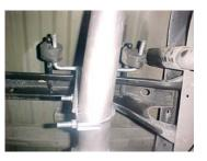
Next install rear muffler hanger# D into grommets just above the outlet of the muffler clamp onto tailpipe. Do not tighten.
