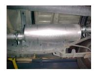
Install muffler #B onto head pipe 1-1/2" to 2" with the louvers facing towards the converter. Use a jack stand to support the muffler. Use clamp #F to secure the muffler to the head pipe. Do not tighten. Muffler inlet is looking into the louvers.
