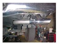
Install the over axle tailpipe # C into the muffler 1-1/2" to 2". Secure to the muffler using clamp #F Do not tighten. Insert welded hanger into rubber grommet.
