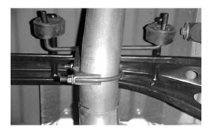
INSTALL REAR MUFFLER OE HANGER #F TO SUPPORT THE TAILPIPE.THE BOLTS FROM THE OE HANGER WILL BE FACING THE DRIVERSIDE. THIS HANGER ATTACHES TO THE TAILPIPE, NOT
