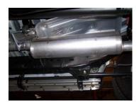
Install muffler #B onto head pipe #A 1-1/2" to 2" with the louvers facing towards the converter. Use a jack stand to support the muffler. Use clamp #F to secure the head pipe. Outlet of muffler will be at the 6 o'clock position.
