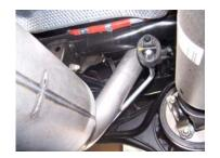
Install the over axle tailpipe #C into the muffler 1-1/2" to 2". Secure to the muffler using clamp #F. DO NOT TIGHTEN. Insert welded hanger into rubber grommet.
