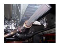
Lay out the exhaust on the floor so it looks like the drawing and compare parts with manual. To remove the stock exhaust remove, it from the 2-bolt flange, just in front of the muffler. Then cut your tailpipe off behind your factory muffler.
