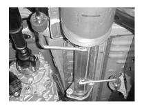
Install head pipe # A on to your existing stock 2 bolt flange. Use hardware kit #G, to secure. DO NOT TIGHTEN.
