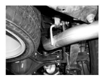
INSTALL THE OVERAXELE TAILPIPE #C INTO THE MUFFLER 1-1/2" TO 2". INSERT WELDED HANGERS INTO RUBBER GROMMET. SECURE TO THE MUFFLER USING CLAMP #E. DO NOT TIGHTEN.
