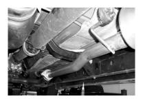
LAY OUT THE EXHAUST ON THE FLOOR SO IT LOOKS LIKE THE DRAWING AND COMPARE PARTS WITH MANUAL. TO REMOVE THE STOCK EXHAUST REMOVE IT FROM THE 2-BOLT FLANGE LOCATED IN THE FRONT OF THE MUFFLER. LEAVE ALL RUBBER GROMMETS IN PLACE. USE WD-40 TO AID IN REMOVAL OF
