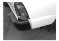
NEXT INSTALL YOUR STAINLESS STEEL TIP TO YOUR DESIRED LOOK. USE ANY ALUMINMUM OR STAINLESS STEEL CLEANER TO POLISH YOUR TIP. MAKE SURE YOU HAVE A MINIMUM OF A 1" CLEARANCE ON ALL PIPES FROM ALL RUBBER BRAKE LINES. TIRES, SHOCKS, FUEL LINES, ETC. THEN **TIGHTEN ALL CLAMPS** AND HANGERS
