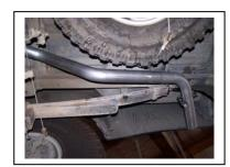
Install the over axle tailpipe # C into the muffler 1-1/2" to 2". Secure to the muffler using hanger # D. Do not tighten.
