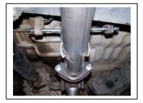
To remove the stock exhaust it, unbolt it at the flange just in front of the muffler and remove stock exhaust. Leave all rubber grommets in place. Use WD-40 to aid in removal of exhaust and hangers.
