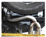
7. Install the exit pipe #D onto the tailpipe. Secure together with clamp #F. Do not tighten. Roll the exit pipe until it is at the correct angle for your vehicle. Insert welded hanger into rubber grommet.
