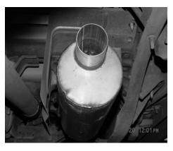
INSTALL MUFFLER # B INTO HEADPIPE AT LEAST 1-1/2" TO 2". USE CLAMP # E TO ATTACH TO THE HEADPIPE. USE A JACKSTAND TO SUPPORT THE MUFFLER. DO NOT TIGHTEN.
