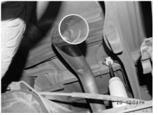
INSTALL OVERAXLE TAILPIPE # C INTO MUFFLER AT LEAST 1-1/2" TO 2" USING CLAMP #E TO ATTACH IT TO THE MUFFLER. DO NOT TICHTEN
