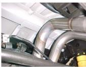
5. Slide driver side over axle tailpipe #C into muffler 1.5-2". Use clamp #G to secure tailpipe to muffler. Do not tighten. Insert welded hanger into rubber grommet.
