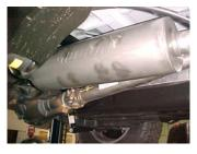
4. Install muffler #B onto headpipe 1½"-2". Use a jack stand to support the muffler. Make sure muffler outlets are level. Use clamp #G to secure the muffler to the headpipe. DO NOT TIGHTEN.
