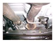
2. To remove the stock exhaust, unbolt it at the 2-bolt flange in front of the muffler. Disengage the welded hangers using WD-40 from the OEM rubber grommets. Do not damage or remove the rubber grommets as you will re-use them to mount your new system.
