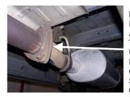
LAY OUT THE GIBSON EXHAUST ON THE FLOOR AND COMPARE PART #'S TO THE DRAWING. UNBOLT STOCK EXHAUST FROM BEHIND CATALYTIC CONVERTER. USE JACK STANDS TO SUPPORT CONVERTER SO IT WILL NOT DROP.
