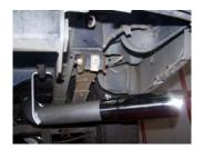
INSTALL THE OVER AXLE TAIL PIPE #C AND ATTACH WITH CLAMP #G AND CONNECT WITH HANGER #E. INSERT WELDED HANGER INTO RUBBER GROMMET.
