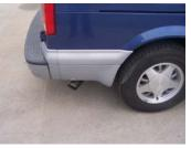
INSTALL STAINLESS STEEL TIP, CLAMP DOWN. NOW TIGHTEN ALL BOLTS AND CLAMPS. TO CLEAN TIP US SCOTCH BRITE AND ANY STAINLESS OR ALUMINIUM CLEANER.
